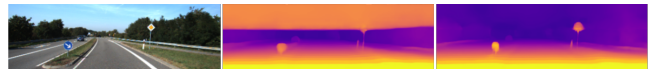
Fig. 2. Depth learning when using standard supervised techniques (middle) may not produce meaningful results for areas of no training data, which is a common problem of applying learning algorithms to real-life systems. Our algorithm counteracts that by combining supervised and unsupervised constraints (right).
