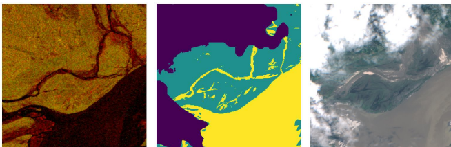
Fig. 10: Sentinel-1 image (left), groundtruth floodmap (middle) and Sentinel-2 image (right) from Sen1Floods11 dataset. Sentinel-2 image is only for visualization and not used during training. Labels include water (yellow), no-water (cyan), and masked out region (purple).
