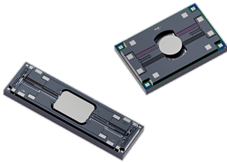
Fig. 1a Optical pictures of electrostatically-actuated, quasi-static (left) and resonant (right) MEMS mirrors fabricated by ST Microelectronics 2,18,19,24,25 (STM) and made of two wafers: A top structural wafer and a bottom handling wafer. (courtesy of STM)
