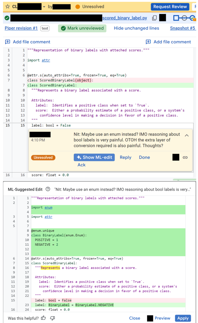
Figure 12: Example: replace a Boolean label with an enumeration, also including relevant imports. Note the conversational language used by the reviewer.
