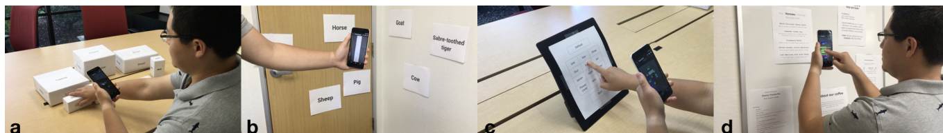
Figure 1. We define and compare cursor-based interactions that support non-visual attention to items within a complex visual scene: (a) window cursor, in which the user moves the device itself to scan the scene and receives information about what is in the center of the image; (b) vertical window cursor, a variation of window cursor that sacrifices the granularity on the vertical axis, but potentially facilitates locating the direction of a specific object; (c) finger cursor, in which the user moves their finger on the real world object they want to access and receives information about details near (or under) their fingertip; and (d) touch cursor, in which the visual scene is brought onto the device screen and the user moves their finger on the touchscreen to receive information about what they touch on the live camera image.
