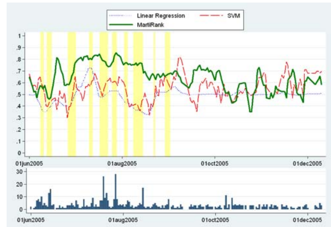
Figure 5: This plot shows the performance of three competing methods (MartiRank, SVM, and linear regression) during the second half of 2005. Each day, we compute each algorithm's performance in terms of the normalized average rank of failures that occurred during that day. MartiRank clearly outperforms the other methods. Further, the periods that are critically important are the peak summer months, when the system is near capacity and feeder failures are more frequent, and these are the periods where MartiRank's accuracy is best. A histogram of daily failure counts is shown below the line graph. All curves in the upper graph have been smoothed using a 5-day moving average for clarity of presentation.
