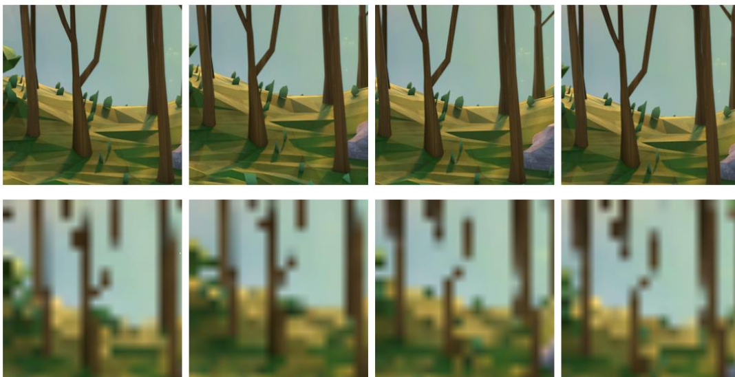
Figure 2. Example of temporal fluctuation. The same content is observed with different shifts, and even though the content is unchanged, the aliasing pattern is dynamic frame-to-frame (4 frames here showing volatile aliasing).
