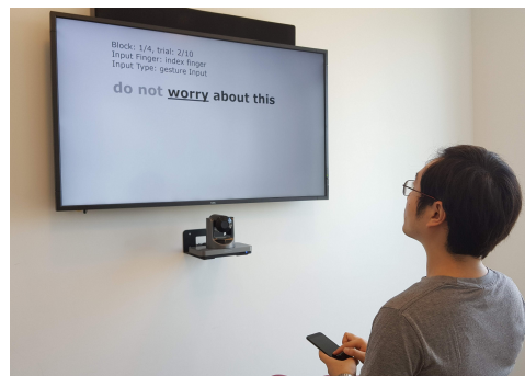
Figure 2: The setup of Experiment 1. A user was seated in front of a TV and performing eyes-free gesture typing.
