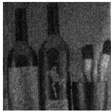
Figure 11. The binary image generated by stitching 1024 binary images taken by the SPAD camera.
