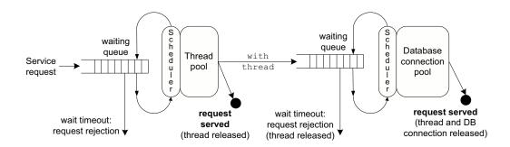
Figure 1. Request execution model with 2-level exclusive resource holding.
