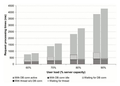
Figure 5. Breakdown of request processing time for the Buy Confirm request (left col.: request-wide database connection caching, right col.: transaction-wide caching).
