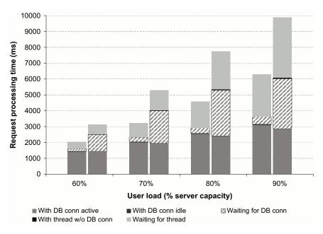
Figure 3. Breakdown of request processing time for the Search request (left column: request-wide database connection caching, right column: transaction-wide caching).
