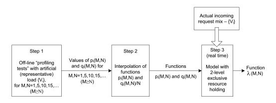
Figure 2. Logical steps of the method to compute the optimal number of server threads and database connections.
