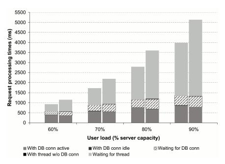
Figure 4. Breakdown of request processing time for the Buy Request request (left col.: request-wide database connection caching, right col.: transaction-wide caching).
