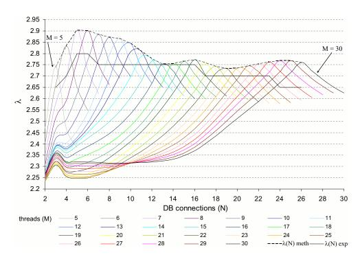
Figure 9.  $\lambda(M, N)$  and  $\lambda(N)$ , computed by our method (" $\lambda(N)$  meth") and obtained experimentally (" $\lambda(N)$  exp"), for the "profiling load."
