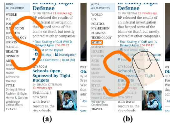
Figure 2: Tapping on a target using Gesture Avatar. (a) The user draws an “S” near the target “SPORTS”. (b) The user taps on the gesture avatar as if tapping on the target.
