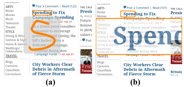
Figure 15: Two different representations we explored for Gesture Avatar: (a) the stroke and (b) the lens representation.
