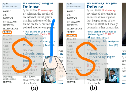
Figure 3: Re-assigning a target to the avatar. (a) The user draws a directional gesture outside the avatar. (b) Gesture Avatar finds the next best match in the given direction.
