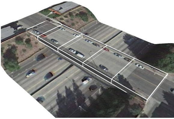
Figure 5: Overpass geometry is approximated with a rectangular prism. Orientation, breadth and elevation are derived from road spans, while the road depth is defined by the user.
