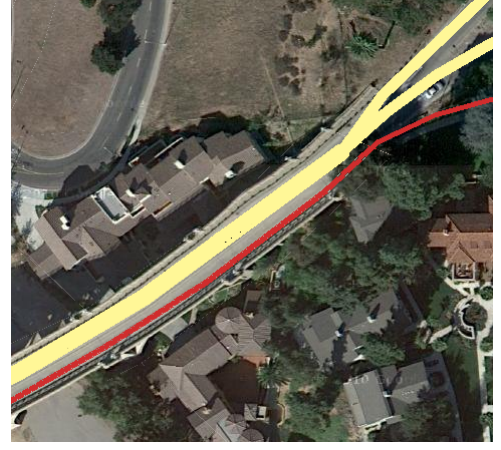
Figure 4: Vector roadways are reconstructed from DSM measurements instead of the original vector data because multiple vector thoroughfares may be sharing the same structure. Here, vehicular (yellow) and pedestrian (red) traffic disjointly share the Colorado Boulevard Bridge in Pasadena, California.
