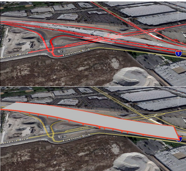
Figure 7: Geometric reconstruction of expanded I-5/Artesia Boulevard overpass structure from older vector road data.
