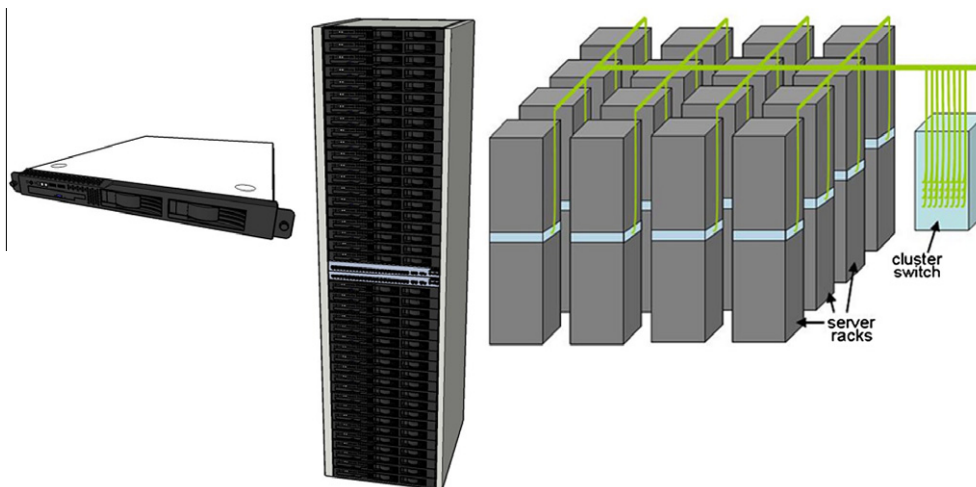
Fig. 1. Typical elements in a Warehouse scale computer.
