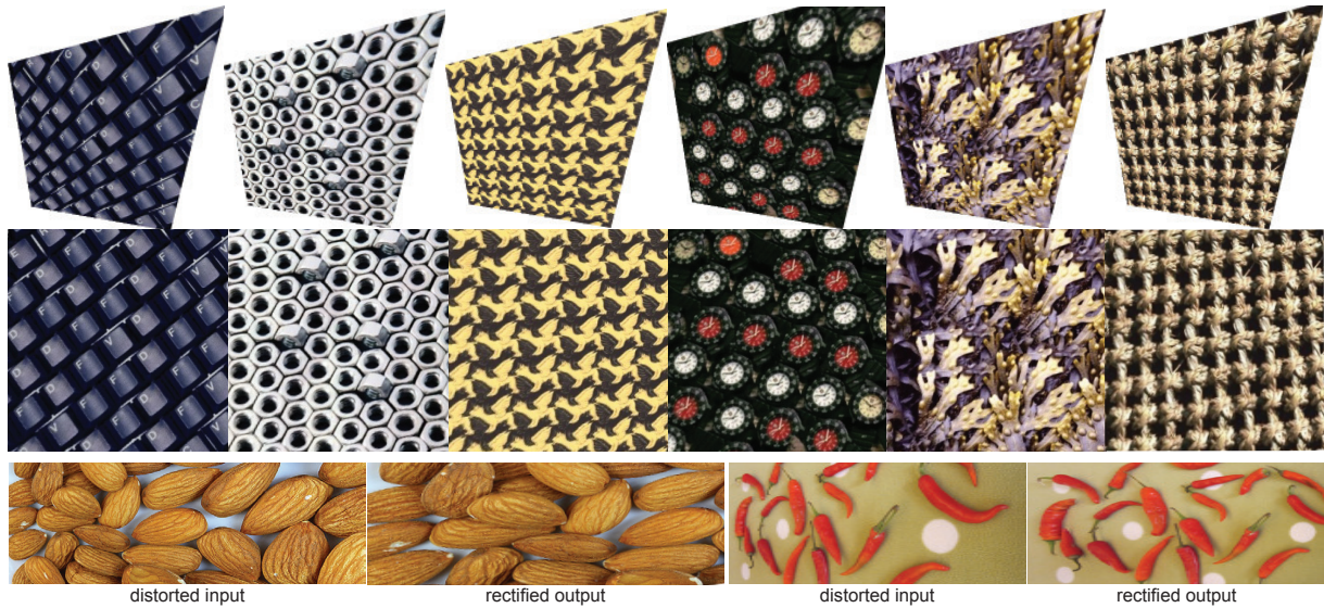
Figure 12: (Top two rows) Automatic unwarping using the proposed algorithm on various well known synthesized textures (source: http://www.cc.gatech.edu/cpl/projects/graphcuttextures/ ). The textures were (synthetically) distorted by the same perspective transform. (Bottom) Rectification results on real-world images. See also supplementary demo and results.
