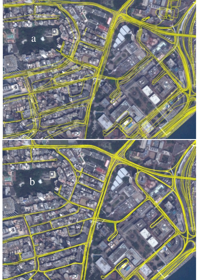
Figure 10. A comparison of vehicle paths in downtown Hong Kong before (a) and after (b) SfM-based correction.
