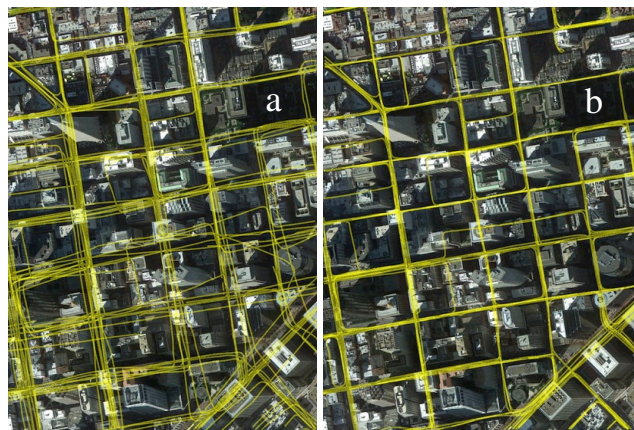
Figure 9. A comparison of vehicle paths in downtown San Francisco before (a) and after (b) SfM-based correction.
