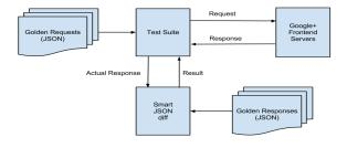
Figure 1. Google+ Mobile Client-Server Test Architecture
