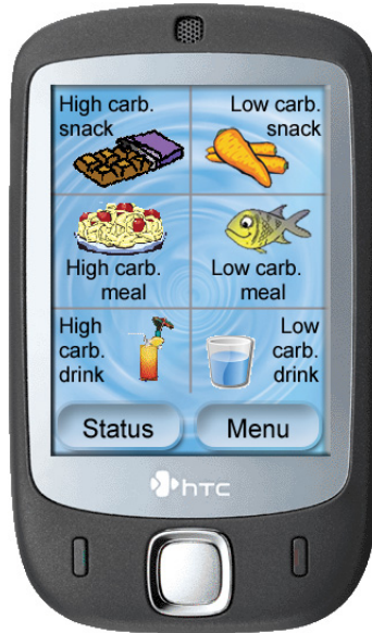
Fig. 2.3 One-touch category-based diet logging in the Few Touch application. The Few Touch application [5] tracks diet with single taps on one of six categories of food and drink.
