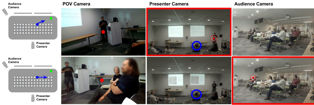
Figure 3. Egocentric FOV localization in indoor environments. The images on the first column show the room layout. The presenter is shown in Green and the person wearing Glass is shown in Blue with his egocentric view shown by the blue arrow. The second column shows the POV video frames from Glass. The red dot shows the focus-of-attention. The third and fourth column show the presenter cam and the audience cam respectively. The localization is shown by the target symbol and the selected camera is shown by the red bounding box. The person wearing Glass is highlighted by the blue circle in the presenter camera views.
