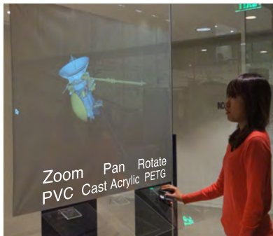
Figure 6: Controller for a floating transparent screen. Different controls (Pan, Rotate, and Zoom) are associated with a set of mouse pads with different transparent materials.
