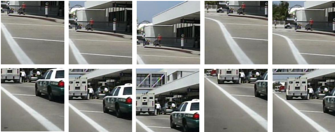
Fig. 2. Procedure for generating examples for training for the LFOV classifier: each of these examples is generated by positioning a pedestrian in the center of each cell of a 4x4 grid, in as many cell positions as possible.
