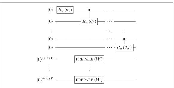
**Figure 1.** The circuit for PREPARE( $\beta$ ) as described in equation (33). An expression for  $\theta_k$  is given in equation (35). PREPARE(W) is implemented using a precomputed classical database.
