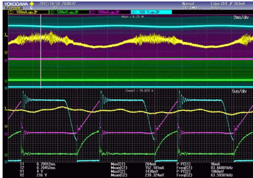
Figure 18 Experimental results at full load (CH1-Yellow: Fan current; CH2-Green: V_{ramp} ; CH3-Pink: I_{Q1} ; CH4-Blue: V_{ds} of Q1)
