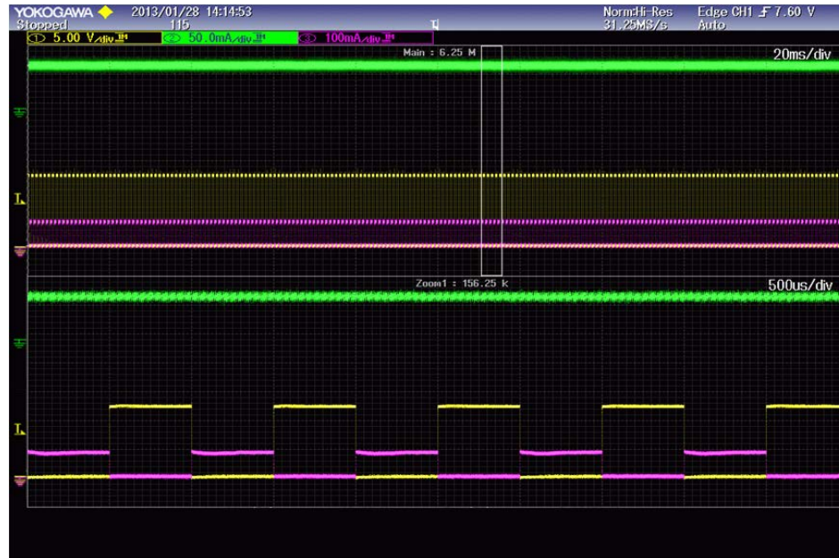
Figure 21 Transient performance during AUX load changes at 1kHz (CH1-Yellow: Control switch voltage of the auxiliary load, CH2-Green: Load current at 70mA, CH3-Pink: Auxiliary load current, 1.2W resistive load+1.8W fan load)
