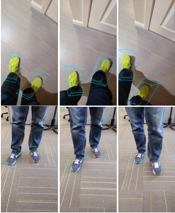
Figure 4: Tracking a 3D bounding box with both camera motion and object movement present.
