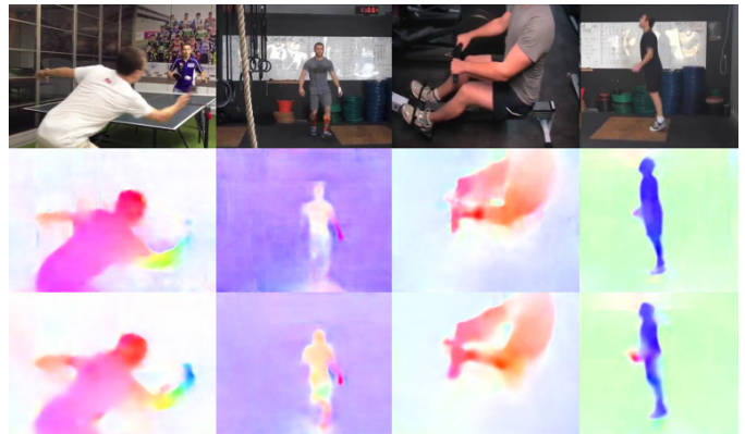
Fig. 7: Qualitative results on QUVA dataset Runia et al. (2018) PWCNet trained on FC (middle) and DMO (bottom). The networks trained using our pipeline capture the non-rigid motion of objects in the scenes with higher detail and delineation. (Best viewed in color.)
