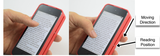
Figure 16: A tactile element represents the current position while scrolling through a document. Touching the element bookmarks the position
