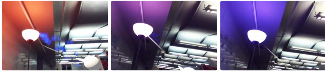
Fig. 8. A sequence of slurping a color from the AR eyedropper to smart lights in the environment. A line from the eyedropper to the target increases the discoverability of the interactive devices. Particle streams indicate the transfer of information between the eyedropper and the target device.
