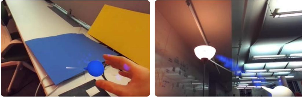
Fig. 7. (a) By using the AR gestural eyedropper to pick up color from real-world environment, the body of the eyedropper changes color based on the extracted color. (b) The emitted color is animated as particles to visualize and represent the intangible process.
