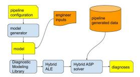
Fig. 1. Diagnostic system architecture.
