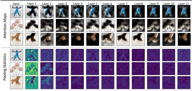
*Figure 4.* Contribution of different layers in Omnidirectional representations for a given set of examples. On top, we plot the omnidirectional attention maps (using OmniNet<sub>B/16</sub>-P12) of one of the heads, over all layers, when CLS token in the last layer is used as query. On the bottom, we show the contribution of each layer to the pooling operation of the Omnidirectional module.
