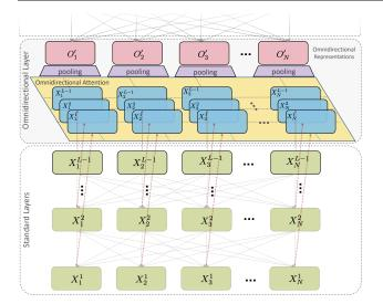
Figure 1. Overview of OmniNet. In the diagram, the omnidirectional module, when partition size is P = L, combines the information across all positions (1:N), across all layers (1:L-1), and for each position selects the best of all layers via a pooling operation to generate the final representations.
