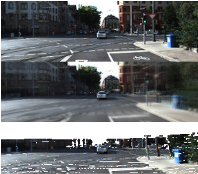
Fig. 2. Comparison of next frame predictions generated by our approach (bottom) with prior work [14] (middle). The input frame is at the top. Trying to predict the RGB values, as it is commonly done, results in a blurry image (middle).
