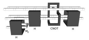
FIG. 22. Uncompute AND (Fig. 4) implemented directly as a Hadamard operation followed by a measurement on the bottom qubit. The outcome of this measurement determines if the sequence of operations on the top two qubits (a CZ implemented as a CNOT framed by Hadamard operations) are included or omitted.
