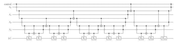
FIG. 7. An L = 11 unary iteration circuit that applies  $X_{\ell}$  to the qubit  $\ell$  in the system register  $|\psi\rangle$ , where  $\ell$  is the value stored in the selection register. The circuit is obtained by merging AND operations from Fig. 5 using the method shown in Fig. 6. It computes 10 AND operations and so has a T count of  $10 \times 4 = 40 = 4L - 4$ .
