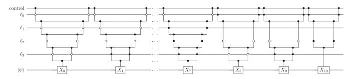
FIG. 5. The "sawtooth" circuit resulting from removing unnecessary bits from Fig. 3 and then adding AND operations from Fig. 4 to combine the controls for performing a controlled indexed  $X_{\ell}$  operation with L = 11 possible targets.
