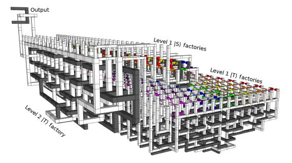
FIG. 24. Preparing a T state in the surface code. Physical  $|T\rangle_0$  states are injected into the 16 lower factories in the lower rear right, which distill them into less noisy  $|T\rangle_1$  states. Fifteen of the successful distillations are forwarded to the larger factory towards the front and left, which distills them into a  $|T\rangle_2$  state with low enough error. The output is shown as the top-left dark U-shape.
