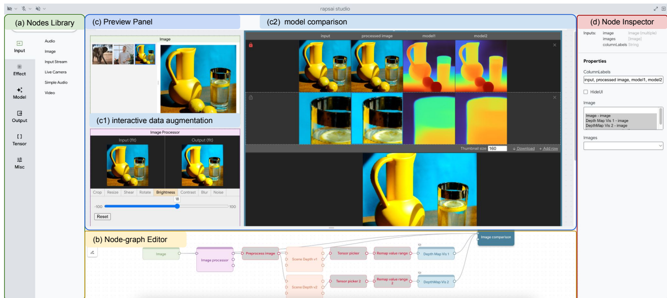
Figure 1: Rapsai is a visual programming platform that empowers machine learning (ML) researchers and practitioners to rapidly build and iterate on real-time ML applications ingesting multimedia data. (a-b) users can build new multimedia pipelines from scratch by connecting input, effect, models, and output nodes within a node-graph editor; (c) users can interactively evaluate the generality of ML models with (c1) interactive data augmentation, and (c2) qualitative comparison to understand the differences and trade-offs between multiple models. (d) In Node Inspector, users can change settings of a specific node, e.g., labels of image comparison. We deploy a public version of Rapsai at http://visualblocks.withgoogle.com
