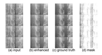
Figure 2: *Example stacked filterbanks from a segment of 3 seconds during training. x-axis is time and y-axis is filterbank.*
