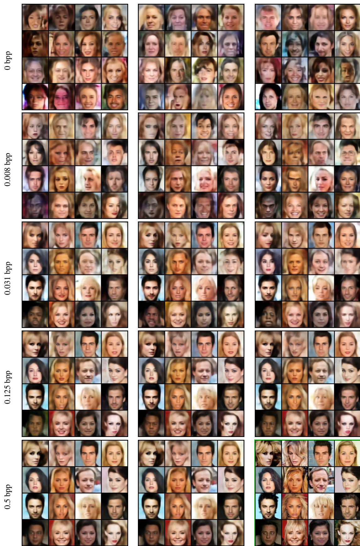
Figure 5: Testing reconstructions produced by our DPLC model with WAE G^* , along with the original image (green border), for CelebA. The variability between different reconstructions increases as the bitrate decreases.
