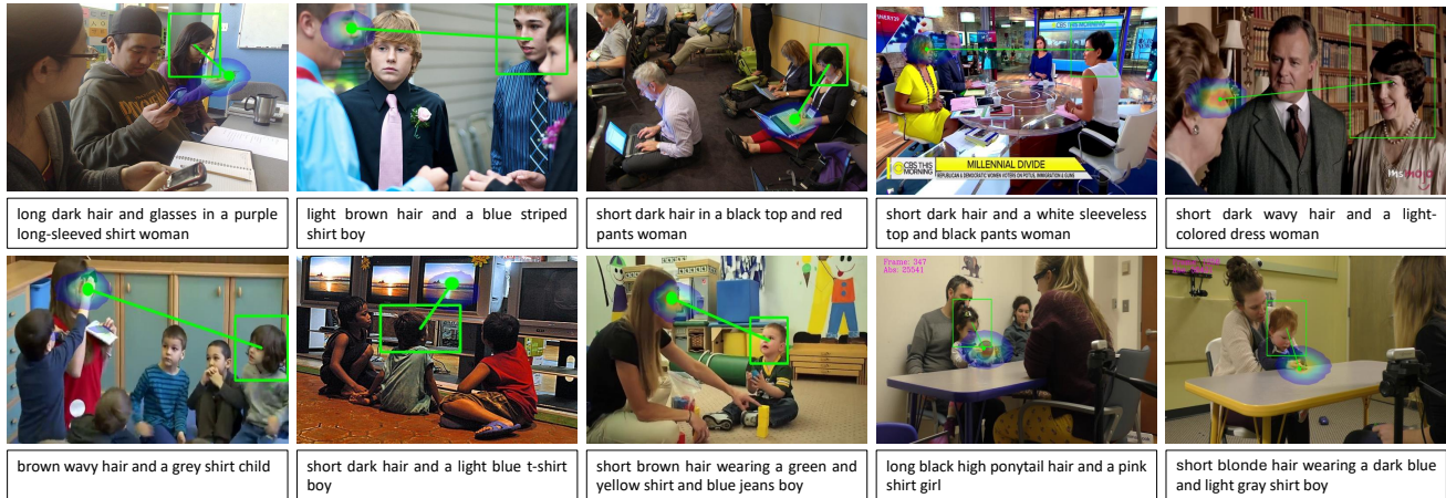
Figure 4. Visualization of AnyGaze’s gaze target estimation results from several datasets. The input is the text prompt (shown in the black box) describing only the subject person’s appearance and the image. AnyGaze detect the subject’s head and track the gaze target. More qualitative comparison is shown in the appendix.
