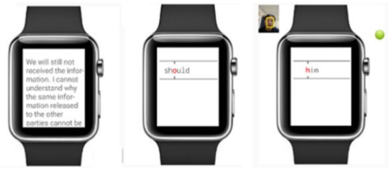
Figure 3. Three reading interfaces in the study. From left to right: Normal Watch Reading (NWR) Interface, Traditional RSVP (T-RSVP) interface, and SmartRSVP.
