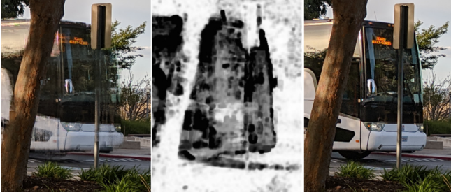
Fig. 9. Motion robustness: Left: Photograph of a moving bus without any robustness model. Alignment errors and occlusions correspond to severe tiling and ghosting artifacts. Middle: an accumulated robustness mask produced by our model. White regions correspond to all frames getting merged and contributing to super-resolution, while dark regions have a smaller number of merged frames because of motion or incorrect alignment. Right: result of merging frames with the robustness model.
