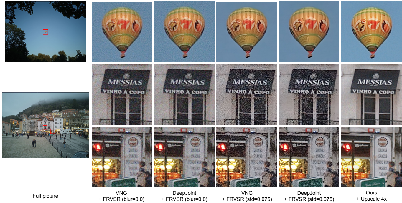
Fig. 15. Comparison with video super-resolution. Our method compared with FRVSR [Sajjadi et al. 2018] applied to bursts of images demosaiced with VNG [Chang et al. 1999] or DeepJoint [Gharbi et al. 2016]. Readers are encouraged to zoom aggressively (300% or more).
