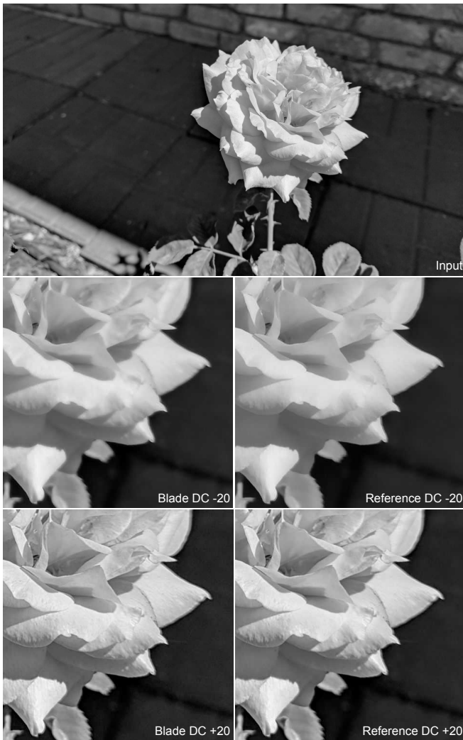
Fig. 9 Example of approximated Detail Control for values -20 and +20 . BLADE has PSNR 38.38 dB and MSSIM 0.9845 for -20 and PSNR 41.36 dB and 0.9895 for +20 .
