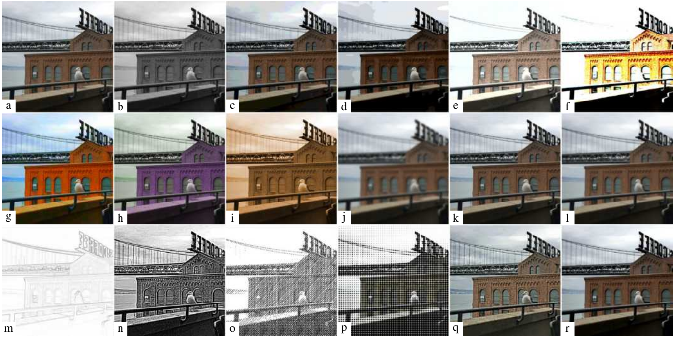
Fig. 4 Filters: (a) Input, (b) To Grayscale, (c) Posterization, (d) Luma Posterization, (e) Brightness, (f) Soft Threshold, (g) Saturation, (h) Hue, (i) Colorize, (j) Gaussian Smoothing, (k) ETF, (l) TVF, (m) Sobel, (n) XDoG, (o) Pattern Filling, (p) Halftone, (q) Image Detail Control, and (r) Linear Equalization. See text for details.
