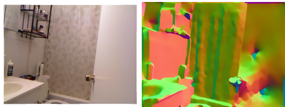
Figure 4: A common example of the errors seen in the normals from [14] that many use for training and evaluation. In these visualizations, (r, g, b) map to (x, y, z) of the normal at that location. Note the oversmoothing, which reduces and removes the normals of small objects. This image also demonstrates why it is important to only backpropagate on pixels that have valid depth, as the right side of the image has incorrect normal data due to noisy and missing depth values.
