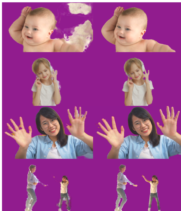
Figure 1. Real-time video segmentation comparison on Google Pixel 6 smartphone. Left column: Baseline ML inference at 89.5% mIoU [2] (segmentation quality metric) and 2.03 Watts. Right column: Our ML inference at 95.1% mIoU and 1.84 Watts.
