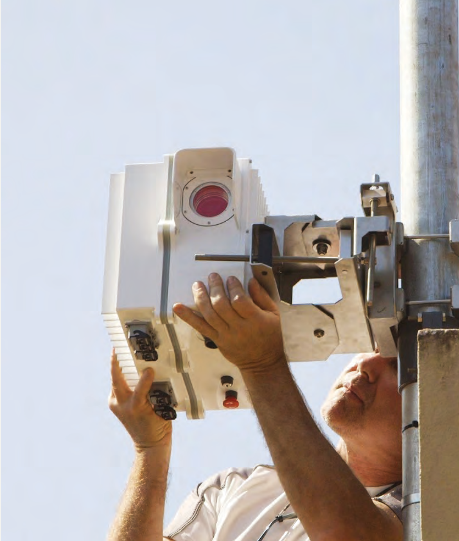
^ A free space optical communications [FSOC] unit is installed for a broadband connectivity test in the Indian state of Andhra Pradesh
