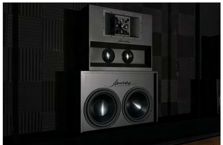
Custom built reduced-depth center channel speakers
