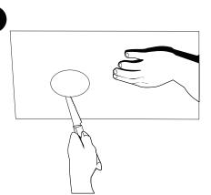
On a free piece of sheet rock cut a hole that is large enough for the sheetrock plug to fit through, yet small enough for the sheetrock trim kit to sandwich the dry wall between the SA assembly (Hole sizing chart below - For your reference).
