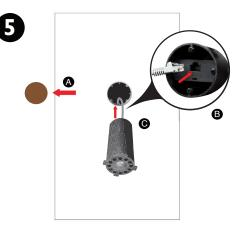
Remove the grille frame plug (A) and connect the SA module to the sub assembly as shown (B). (We recommend using a twisting motion when inserting the SA module (C). This prevents the cable from bunching up and obstructing the port when the module is inserted.)
