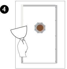
Use mesh tape to cover any installation seams. Insert the grille frame plug before applying joint compound. Apply joint compound and level out compound to conceal seams.
