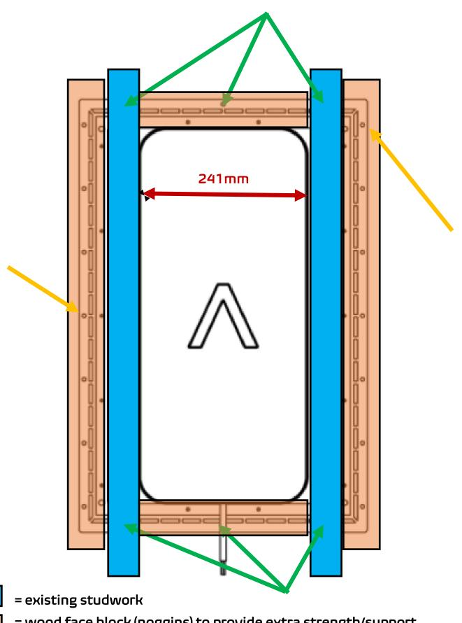
= wood face block (noggins) to provide extra strength/support
