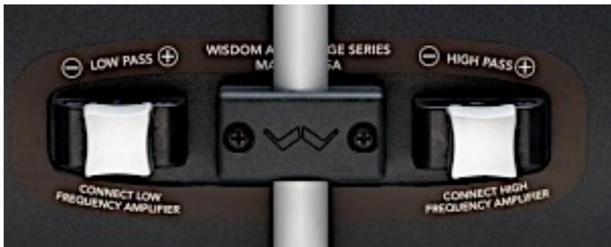
Connect the outputs of your Wisdom Audio SA-series amplifier to the appropriate woofer sections, taking care to get both the channel assignments and the polarity correct. Connect the positive (+) terminals on the SA Series amplifier to the positive (+) terminals for the woofer on the loudspeaker; likewise, connect the negative (-) terminals on the amplifier and the speaker, respectively.
