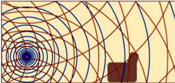
By contrast, the Sage L150m speakers radiate sound as a “line source”. The sound moves into the room as an expanding cylinder, rather than as an expanding sphere — as though from a vertical line suspended in space.
