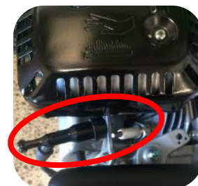
Disconnected spark plug
