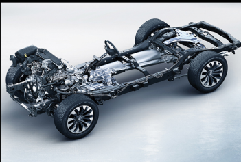
Professional off-road suspension and body-on-frame chassis
