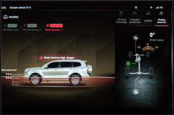
Wading Depth Detection Water depth detection system
