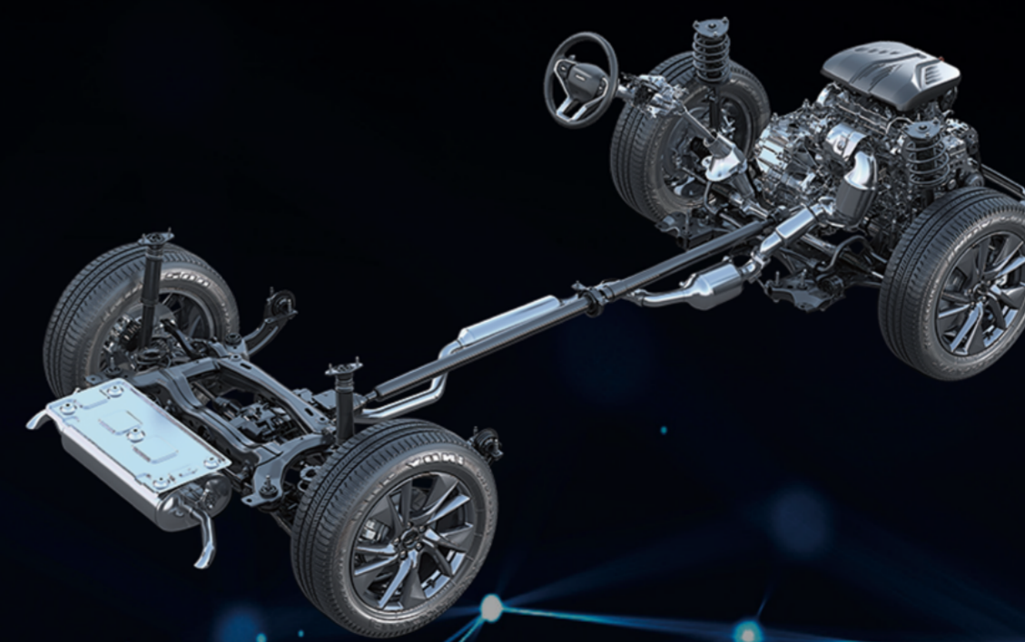
▶ Front Macpherson rear multi-link independent suspension + AWD
