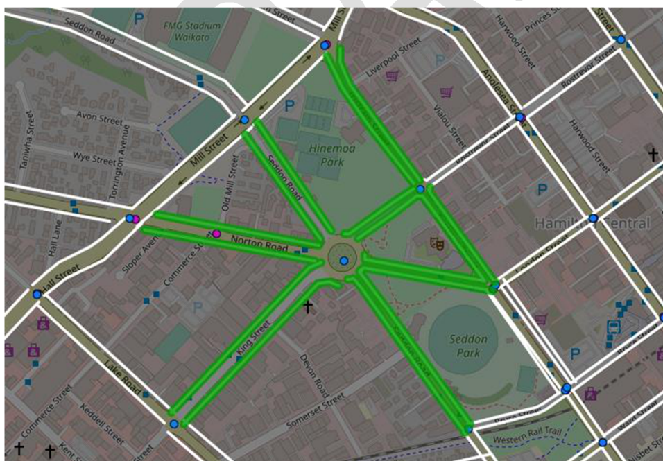
Figure 13 Road links where travel times were analysed (shown in green) before and during the closure of Rostrevor Street between Norton Road and Tristram Street
