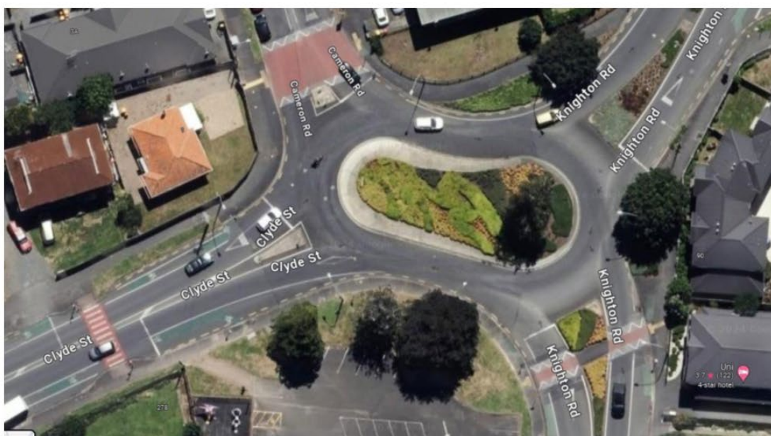
Peanut roundabout at Knighton Road, Clyde Street and Cameron Road intersection, Hamilton
